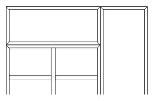
Note: Depth based on 1-1/2" glass thickness for interior installation. Add 3/4" for exterior applications.
