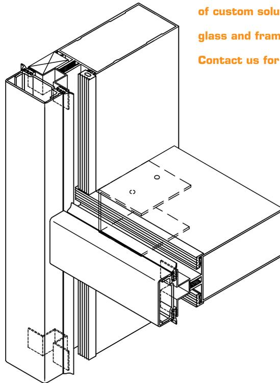
**Note: Depth based on 1" glass thickness for interior installation.**
